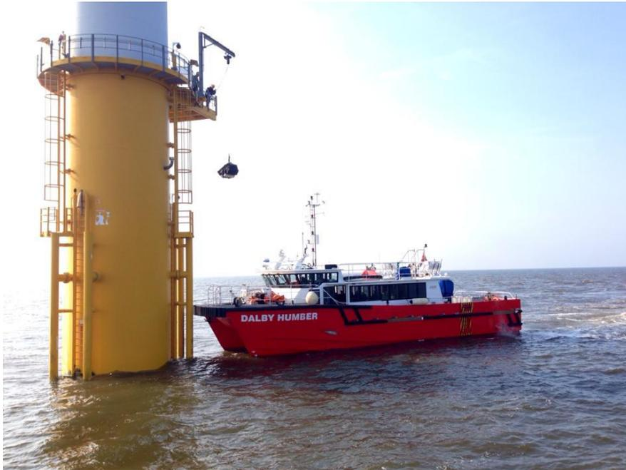
Typically, vessels are between 15 and 30 m in length and up to 8m beam and a draft of between 1 and 2m
